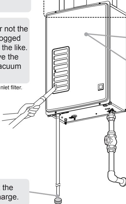
**Check** For blockage at the drain pipe discharge.
