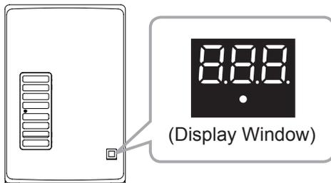
The display window allows you to view the status of unit or error codes.
