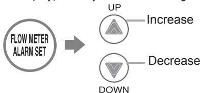
Choose the flow meter alarm setting from the following options: 10 - 60 gallon (40 - 240L) (In 5 gallon (20L) intervals), 70 gallon (260L), 80 gallon (300L), 90 gallon (340L), 100 gallon (380L), 990 gallon.
