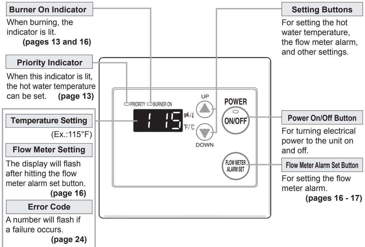
\* Before use, remove the protective sheet from the remote controller surface.
