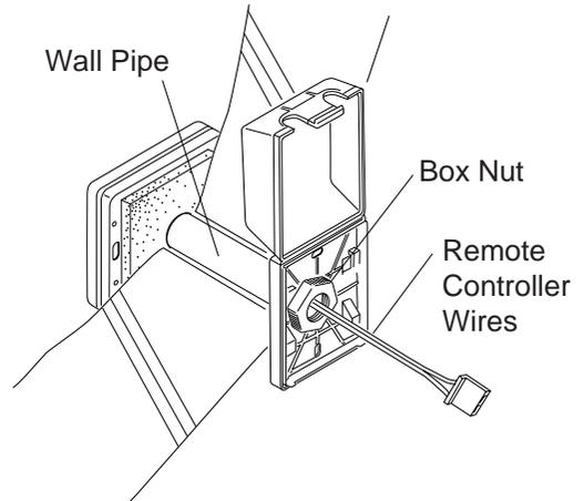
2. Drill a  $\phi 1\text{-}1/4\text{'}$  hole in the wall where the remote controller will be installed.
