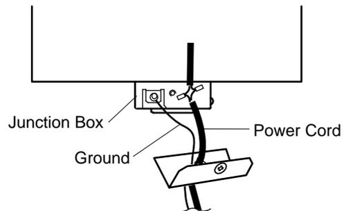
1. Remove the screw (one) of the junction box and open the cover of the junction box.
