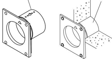
Waterproof the clearance between the sleeve and wall hole with a high temperature sealant.
