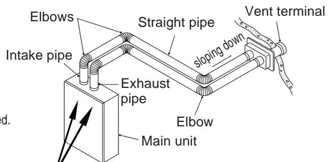
Use a listed Category III vent adapter to connect the flue collar to the vent system. Use Category III vent pipe for the entire length of the exhaust pipe.
