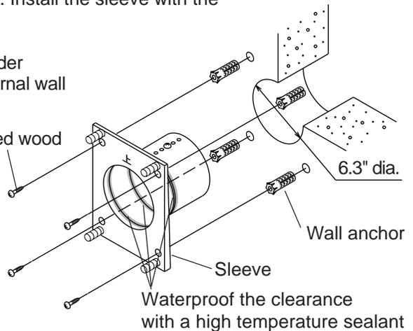
Waterproof the clearance with a high temperature sealant
