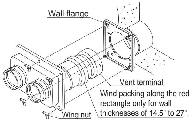
\* Installation pattern (3) yields a clearance between the vent terminal and the wall surface. Fill this clearance with a high temperature sealant.
