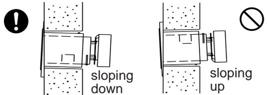
3) Install with the proper length protruding through the wall
